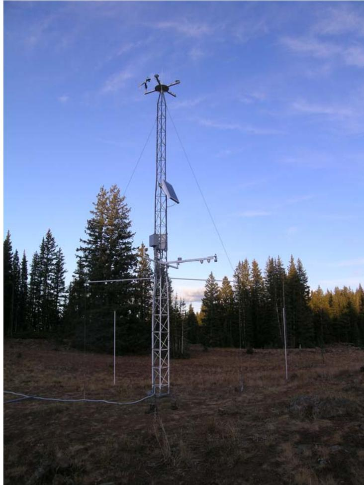
*Figure 3 – the new Grand Mesa Study Plot snow albedo monitoring instrumentation array just after startup, on October 18, 2009.*
